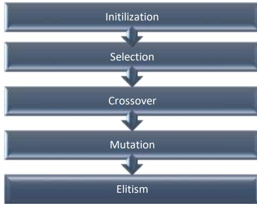
Figure 4. 1 Genetic Algorithms Flowchart Stages
